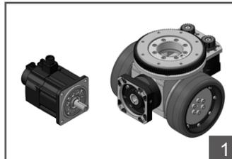
Verify that the motor model and reducer specifications are correct. Also, clean the mating surface.
