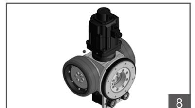
Install and securely tighten the screw plug to prevent small objects from entering the reducer.
