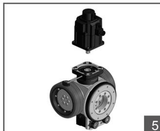
Install the motor vertically into the reducer.
